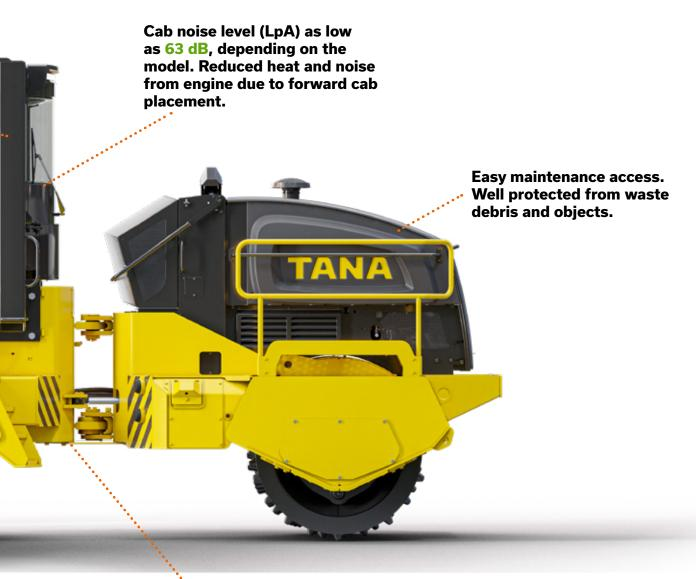
High ground clearance of 840 mm eliminates the need for belly pans.
