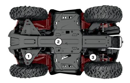
Our Plastic Plates glide smoothly and silently over obstacles, offering great protection in rough terrain. Made of 1/4" (6 mm) thick abrasion-resistant thermoformed High Molecular Weight Polyethylene (HMWPE).
